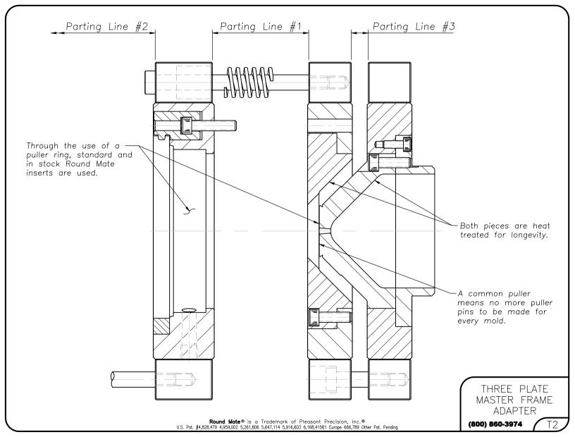
Self contained bars allow all three plate components to be housed out side of the base. This allows for faster adjustments to the plate seperations.
